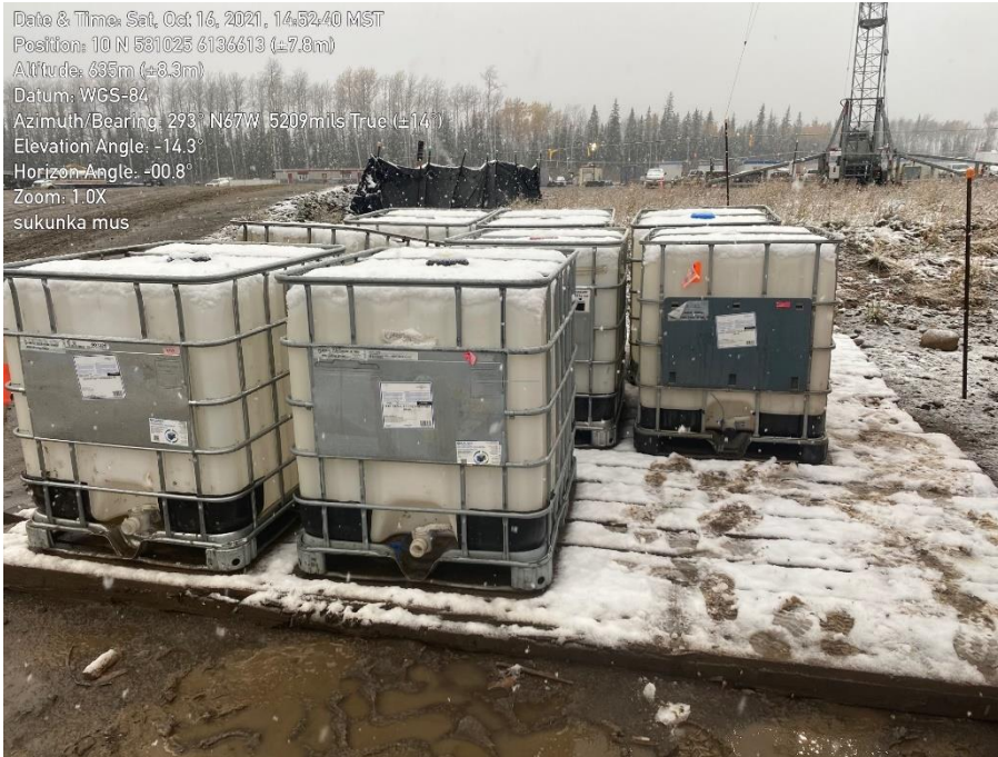
Photo 25. Bulk containers, label indicates they contain diesel engine oil, without secondary containment at Sukunka MUS.
