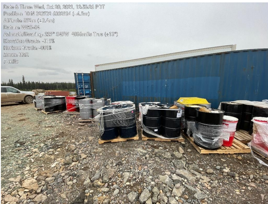
Photo 29. Bulk chemical liquids stored without secondary containment- 7-mile laydown.
