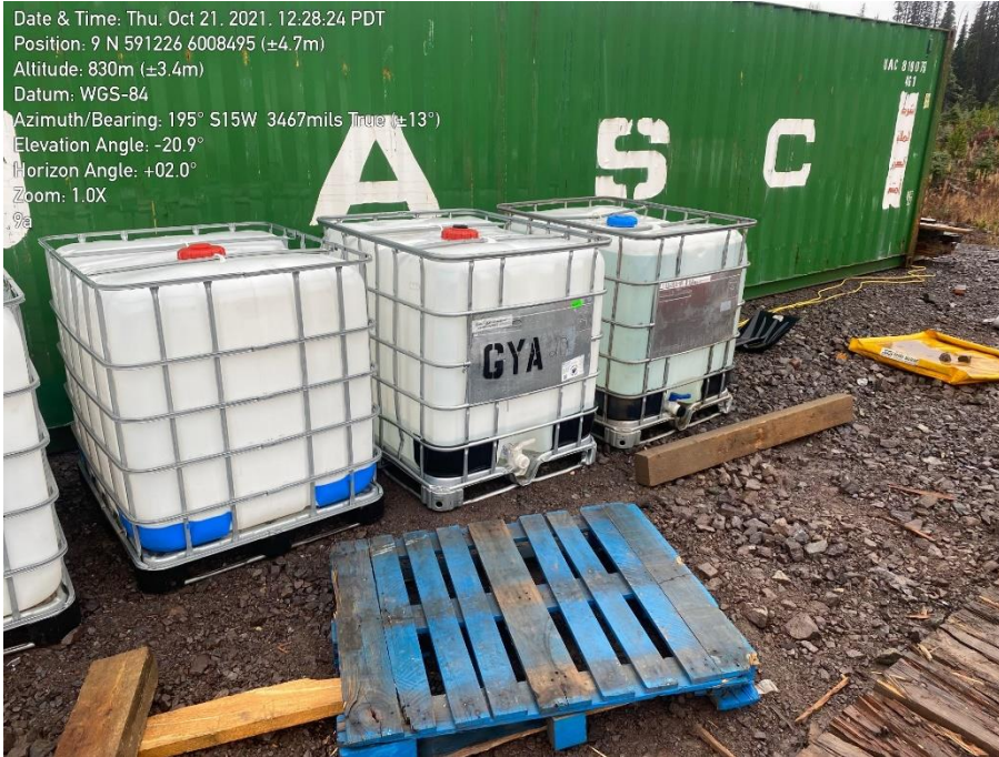
Photo 30. Unlabelled bulk containers without secondary containment beneath.
