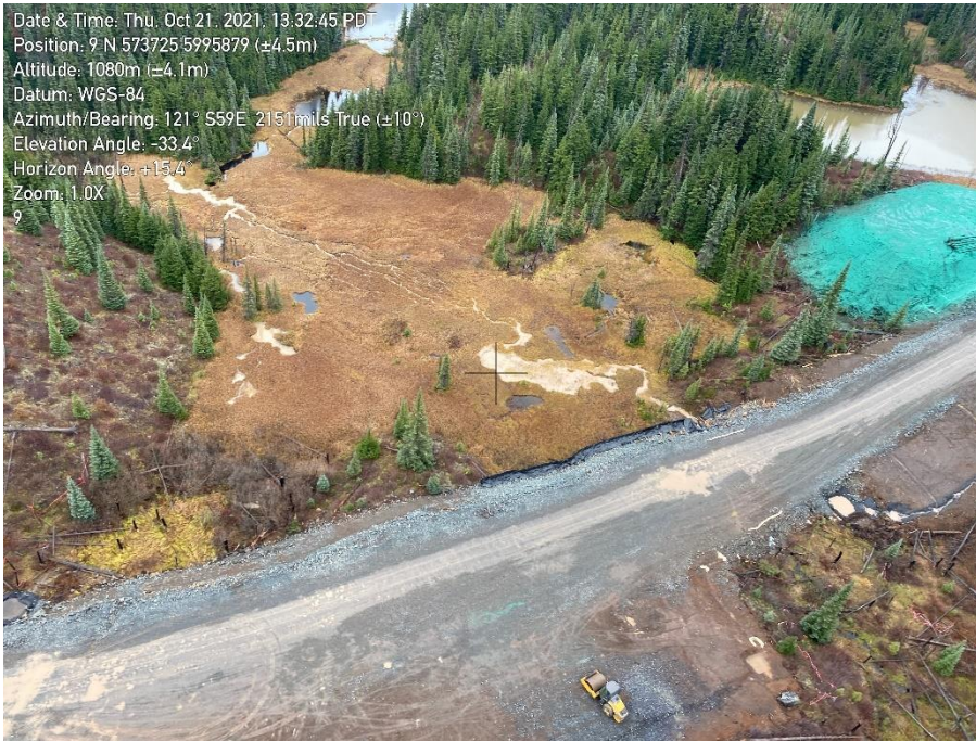
Photo 10. Near KP 600+050. Sediment laden water leaving ROW and discharging to wetlands downslope.
